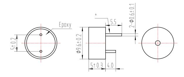
Unit: mm Tolerance: ±0.5mm Except Specified
