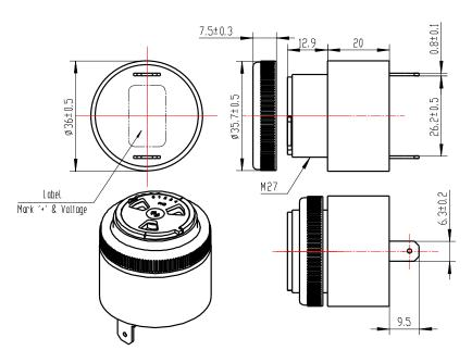
Unit: mm Tolerance: ±0.5mm Except Specified
