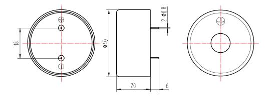
Unit: mm Tolerance: ±0.5mm Except Specified
