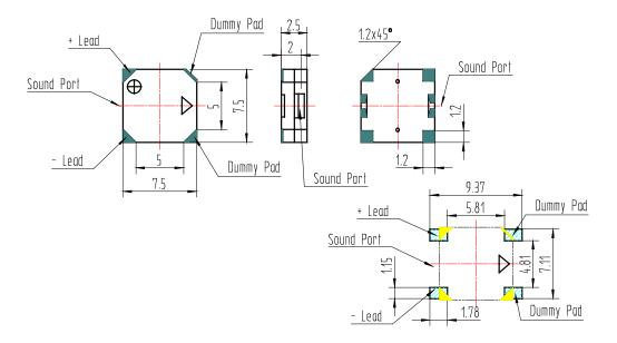
\*Unit: mm; Tolerance: ±0.3mm Except Specified
